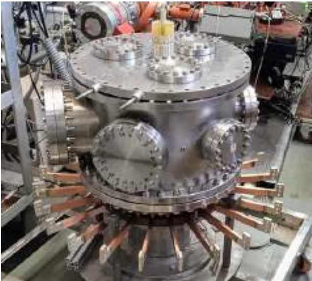
Figure A.2.7: Newly fabricated SMARTEX-C vacuum chamber along with toroidal field coil bus-bars, and support structure.
