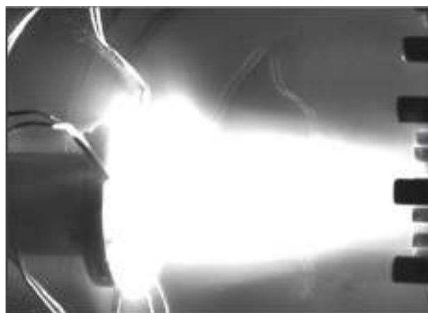
Figure A.1.20: One of the hydrogen plasma beam stream interactions with the copper block of calorimeter.
