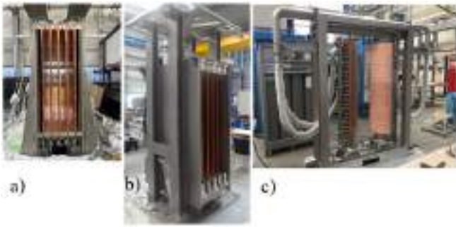
Figure B.1.6: DNB beam line components a) neutraliser, b) RID, c) calorimeter.
