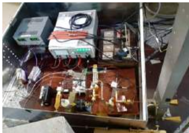
Figure A.3.11: Schematic block diagram and 100 GHz heterodyne system.
