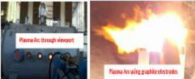
Figure A.1.5: 100kW plasma arc system.
