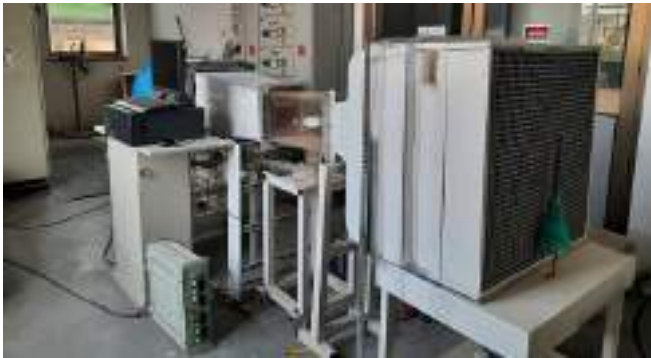
Figure A.1.21: In-house developed subsonic wind tunnel for drag reduction experiment.
