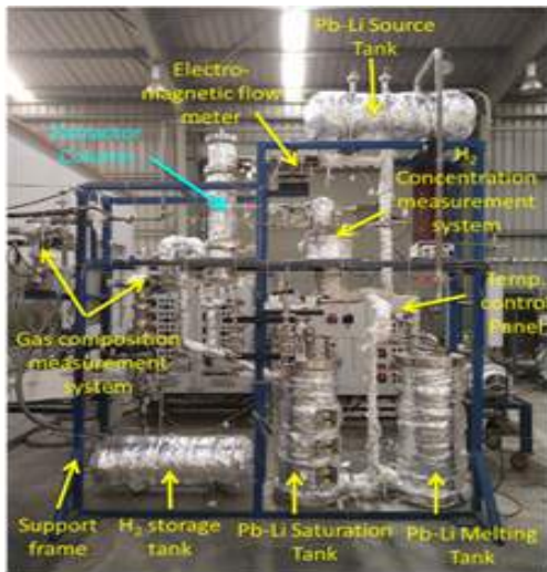
Figure A.4.12: Installed HIES set-up.
