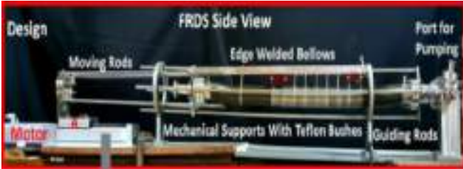
Figure A.3.4: A view of Fast Reciprocating Drive System (FRDS).
