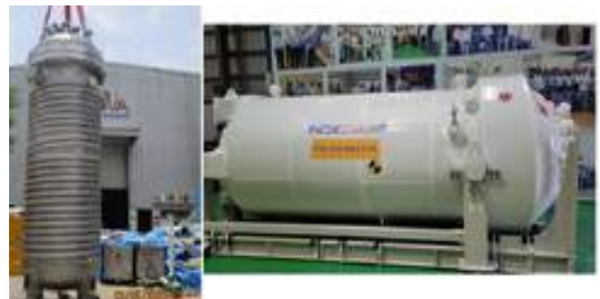
Figure B.1.3: Pool scrubber tank PST under lifting test and packed for shipping at the manufacturer’s site.
