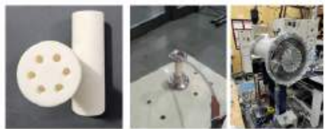
Figure A.4.20: Development of post insulators with insulator metallic flange bolted concept and HV testing.
